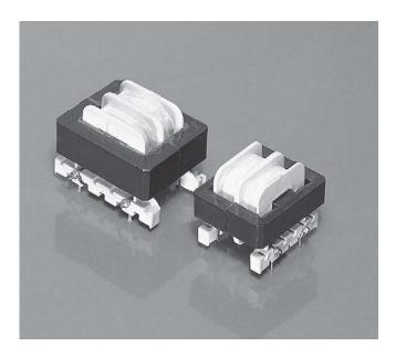
Coilcraft common mode standard packages incorporate several features to help meet the requirements of all major international safety agencies. These include 2 mm thick center flanges and 3 mm creepage and clearance from all terminations to the core.
